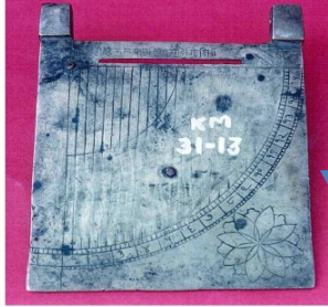
Figure 2: Dhruva/brama-yantra, made for Yado Joshi, resident of Ukala-grāma (Akola), latitude 20 degrees. Reverse side, with the sine quadrant. Raja Dinkar Kelkar Museum, Pune.
