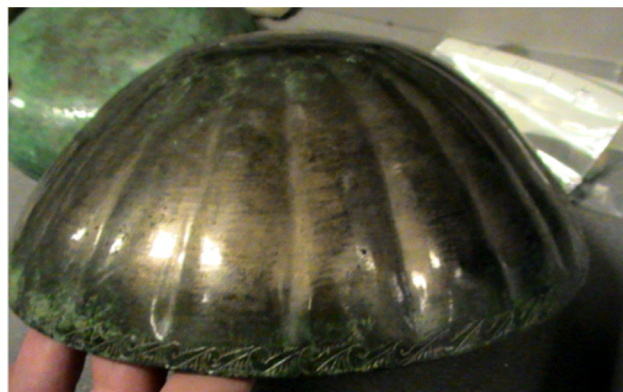
Fig. 12. Beta high-tin bronze vessel from Nilgiris with fluting and striations indicating it was polished using a hand lathe
