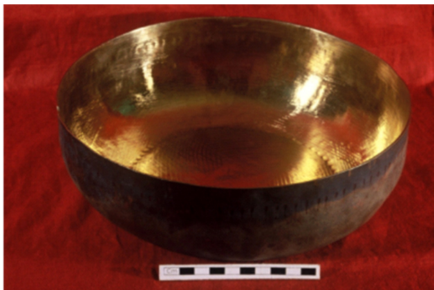
Fig. 7. Wrought and quenched high-tin bronze bowl made in Payangadi in 1991 with 23% tin
