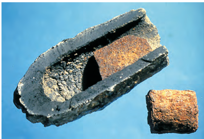
Fig. 12. Broken crucible steel mould, 19 th century from Mawalgaha, Balangoda, Sri Lanka (BM OA Reg. 2002, 1-31, 3), with a typical contemporary steel piece alongside and another inserted back inside
