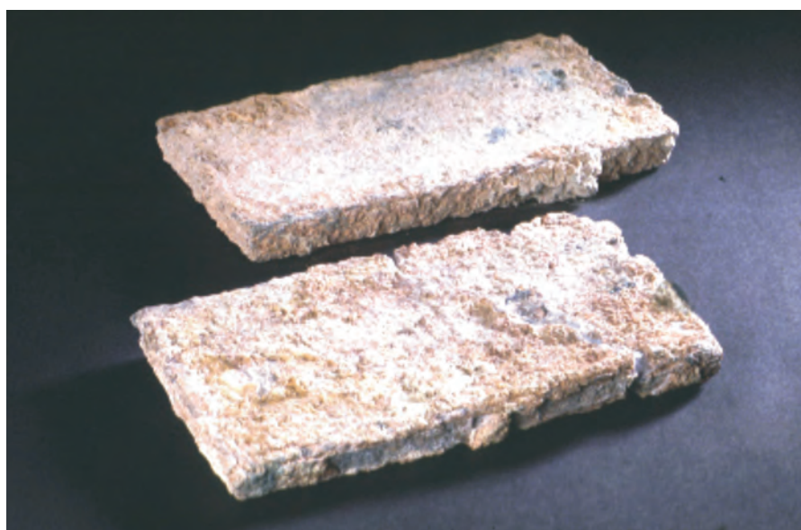
Fig. 11. Typical Chinese zinc ingots from the EIC Diana , wts. 0.7 & 0.8 kg, wrecked off Malacca, Malaysia in 1816, enroute to Calcutta. Dick Lauder (1820) recorded that Chinese zinc was sent to India in plates approximately 8 or 9 inches long by 5½ inches wide and 5/8 thick (20-23 cm × 14 cm × 2 cm, almost identical to those in the plate illustrated here) (BM PE Reg. 1997, 2-2, 1 & 2).
