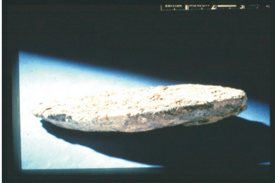
Fig. 4. Typical Chinese zinc ingot, wt. 2.5 kg, from the VOC Witte Leeuw wrecked off St. Helena in 1613. (BM PE Reg. 1990, 12-4, 1)
