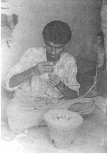
Fig. 25. Artisan fixing the object to be polished on the stick fixed with wax.
