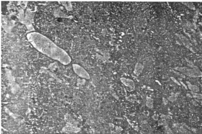
Fig. 19: Black spots developed due to shrinkage during solidification, 200x.
