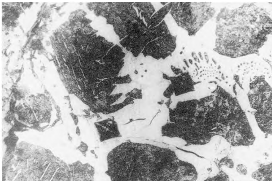
Fig 4. Micro Structure consists of cementite (white), fine pearlite (Black) and ledeburite. Micro hardness impressions can be observed. 280x
